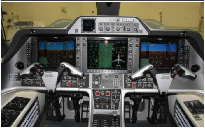
Embraer's Prodigy™ Flight Deck with Garmin's G1000 Integrated Instrument and Avionics System All-glass Avionics Suite includes:
